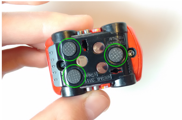
Figure 4.2: The underside of the AppMATes widget has three detection points (indicated with green circles) as well as three lenses that are used to capture light from the screen and project it out to simulate car headlights.
